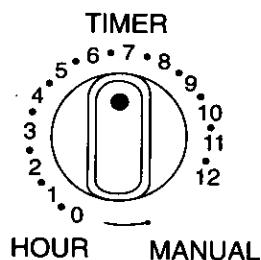
When you turn the Timer Control knob to the MANUAL setting, the air conditioner starts immediately and operates continuously if the Main Control knob is at any setting other than OFF.
