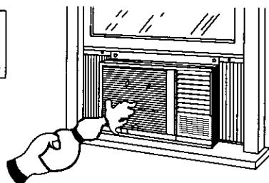
Do not splash water or detergent into the unit's body openings.
