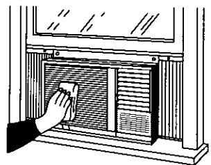
3. Rid the rear air inlets of dust by using a paint brush, or the like.
