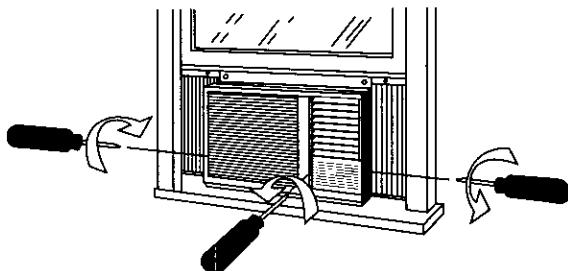
3. Pull the front grille towards yourself from the bottom first, lift up and remove it.
